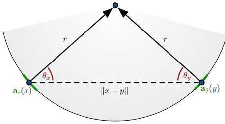
**Figure 1:** The form factor geometry for a spherical dome.
