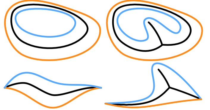
Fig. 10. Geometrically valid configurations (left) and invalid ones (right), with bifurcations of the medial axis, are shown for disjoint loops (top) and for quasi-disjoint strokes (bottom).
