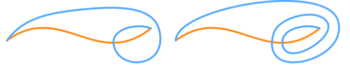
Fig. 5. Invalid configurations with winding number greater than one.
