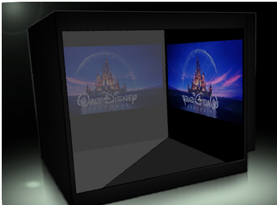
Figure 5. A rendering of the dual-monitor stereo device shows left and right monitors with beam-splitter glass between. Notice the right eye image is flipped horizontally. Image copyright 2010 Disney Enterprises.
